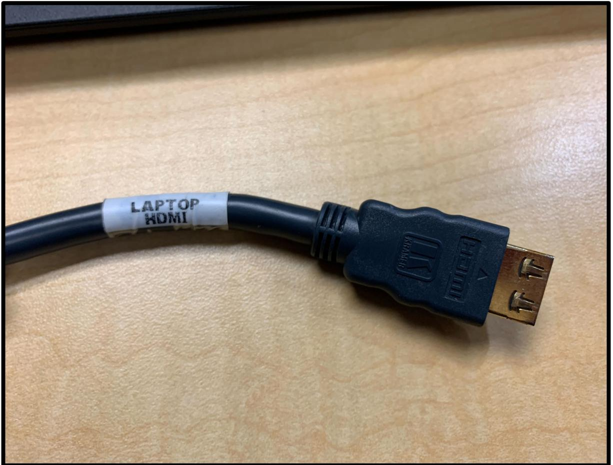
Locate the podium HDMI cable with the label "LAPTOP HDMI". This is the correct HDMI cable for devices that you want displayed onto the room projectors with or without device audio.
